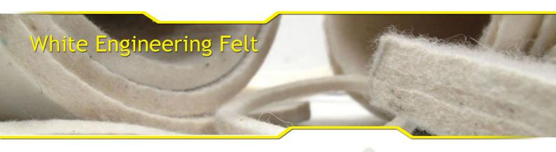
Engineering felt has a vast variety of uses. We mainly use it for sealing and lining in the engineering sector.
