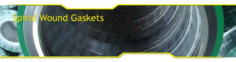
Spiral-wound gaskets comprise a mix of metallic and filler material. Generally, the gasket has a metal wound outwards in a circular spiral wound in the same manner but starting from the opposing side. This results in alternating layers of filler and metal. The filler material in these gaskets acts as the sealing element, with the metal providing structural support.
