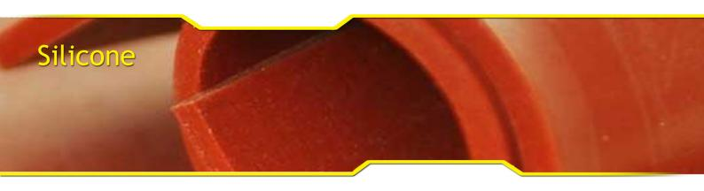
At extreme temperatures, the tensile strength, elongation, tear strength and compression set can be far superior to conventional rubbers. This makes it one of the materials of choice in many extreme environments.
