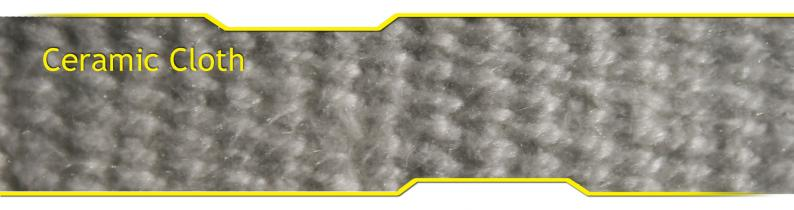
Ceramic Cloth is a woven fabric that is manufactured from high purity ceramic fiber, reinforced with fiberglass filament and optional alloy steel wire.
