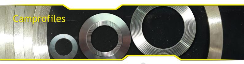
Camprofiles are a composite gasket, which utilises a serrated metal core with a soft facing material. The metal core is machined on each contact face with concentric serrations which provide high pressure areas, ensuring that the soft coating flows into any imperfections in the flange even at relatively low bolt loads.
