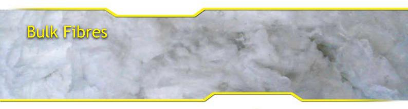
Ceramic fibres are manufactured from aluminosilicate materials and are chemically inert.
